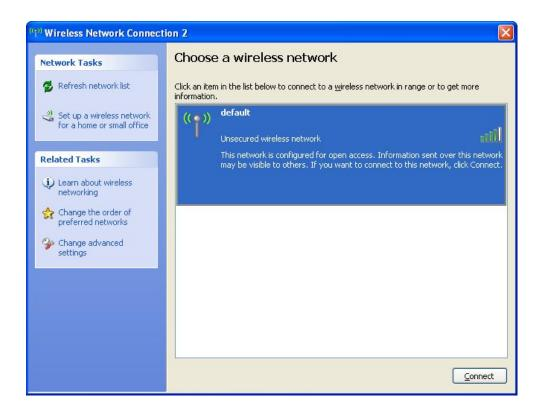
**Step 6.** If the wireless access point uses encryption, users will have to input the correct WEP passphrase or WPA pre-shared key. Ensure both the AP and PC is set with the same WEP passphrase/WPA pre-shared key. Otherwise the wireless connection will fail to establish.
